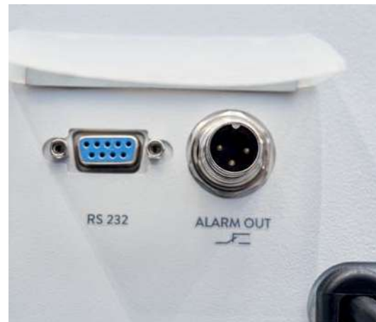
Standard-issue RS-232 interface and alarm contact
