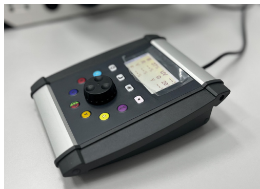
The Viluma 5/7 light control console offers flexible switching across LED wavelengths with precise intensity adjustment.
