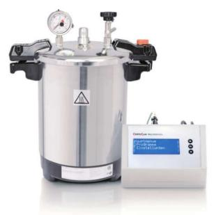
The sterilization chamber is made of high-quality 3103 aluminum. A heater is pressed into the bottom of the chamber, but the heating elements do not get into contact with the water directly and therefore cannot calcify. This extends the service life of the autoclaves. Furthermore, our autoclaves are extremely low maintenance.
