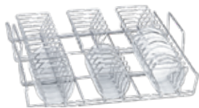
E 118 insert 1/1 for the optimum loading of 38 half petri dishes with Ø 100 mm. Equipped with 38 holders, height 70 mm, distance approx. 26 mm
