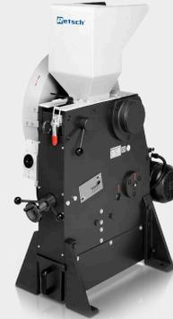
**The Jaw Crusher BB 200 is a floor model designed for a throughput of up to 300 kg/h, suitable for many typical crushing tasks. It accepts feed sizes up to 90 mm. The gap width can be set stepless from 0-30 mm.**
