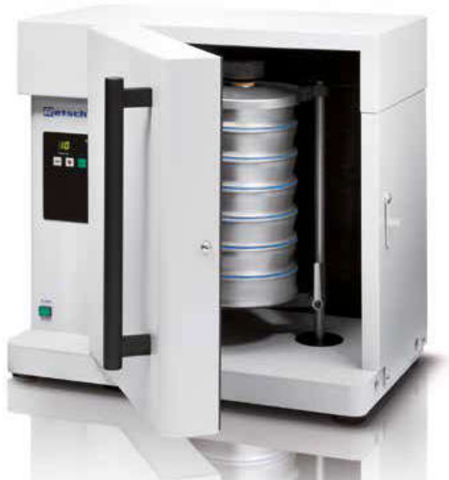
AS 200 tap with sound-enclosure cabinet and sieve stack
