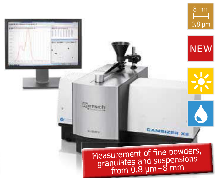
CAMSIZER X2 with X-Jet module for dispersion by air pressure
