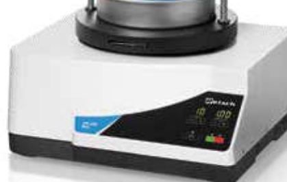
AS 200 basic with clamping device "economy" and sieve stack
