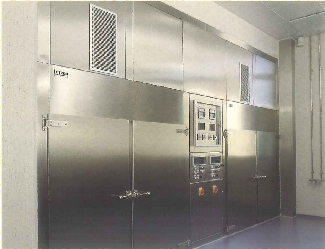
Two granulate dryers type E with common control board for controlling and recording of temperature, solvent and time
