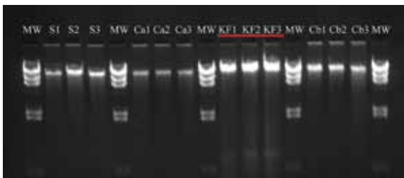
FIGURE 5. In the comparison between different purification processes, the highest yield of gDNA was obtained with the KingFisher Blood DNA Kit (S1 = spin column, Ca = competitor magnetic particle kit, KF = KingFisher, Cb = competitor purification automate).
